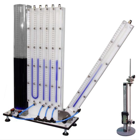
Equipment designed for the study of fluid static and pressure measurement with different types of piezometric tubes and level measuring elements such as graduated scales and limnimeter.
